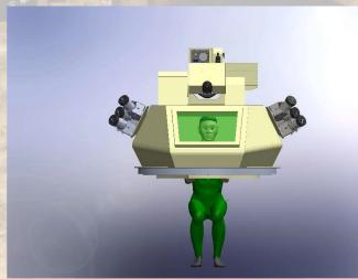
The Terminator 30 is a closed turret with level 2 protection for rapid target engagement at short ranges. The purpose of the Terminator 30 system is to provide defensive firepower for the vehicle crew with level 2 protection for the operator to enemy shell fragments and small arms fire.
